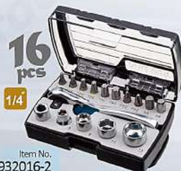
16pc 1/4"DR. Smart-Profile Socket set 4- Low-profile Sockets: 6, 8, 10, 13mm. 2- Accessories: Stubby Ratchet KH3300 AIR, Coupler for bits. 10- Bits (1/4"x25mm): PH#2, 2. Hex: 5, 6mm. TX: T-10, 15, 20, 25, 30, 40.
